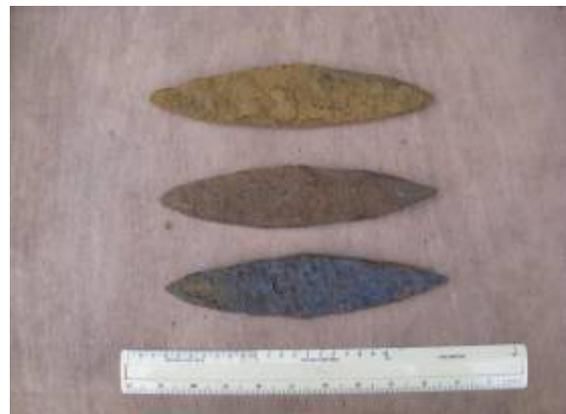
**Fig 3. Pick blades for dressing the mill stones.**
